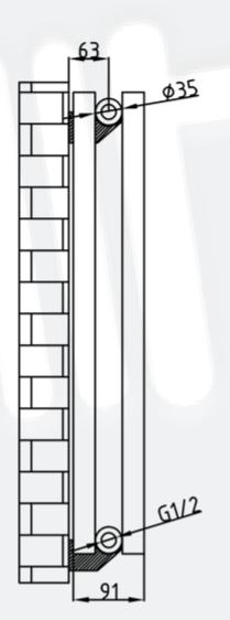
All Direct Radiators are BOE and pipe centres are the radiator width plus 74mm.
