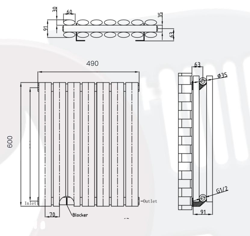
All Direct Radiators are BOE and pipe centres are the radiator width plus 74mm.
