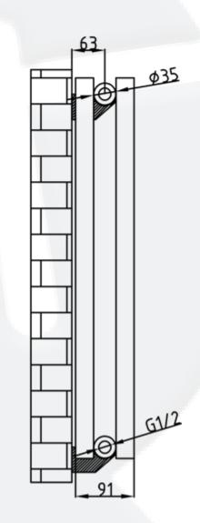
All Direct Radiators are BOE and pipe centres are the radiator width plus 74mm.
