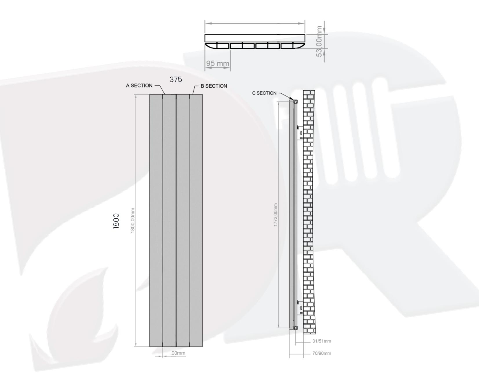
All Direct Radiators are BOE and pipe centres are the radiator width plus 74mm.
