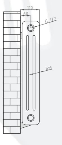
All Direct Radiators are BOE and pipe centres are the radiator width plus 74mm.
