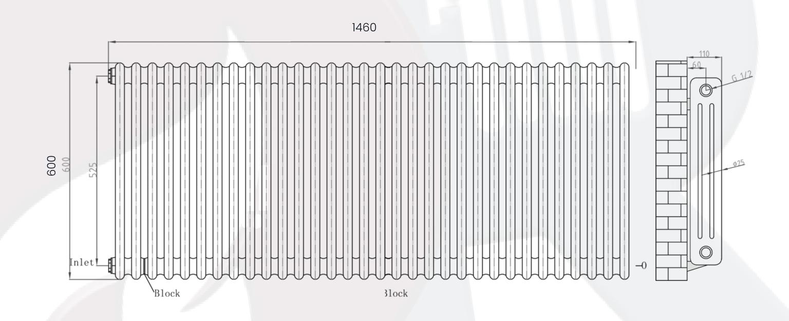
All Direct Radiators are BOE and pipe centres are the radiator width plus 74mm.
