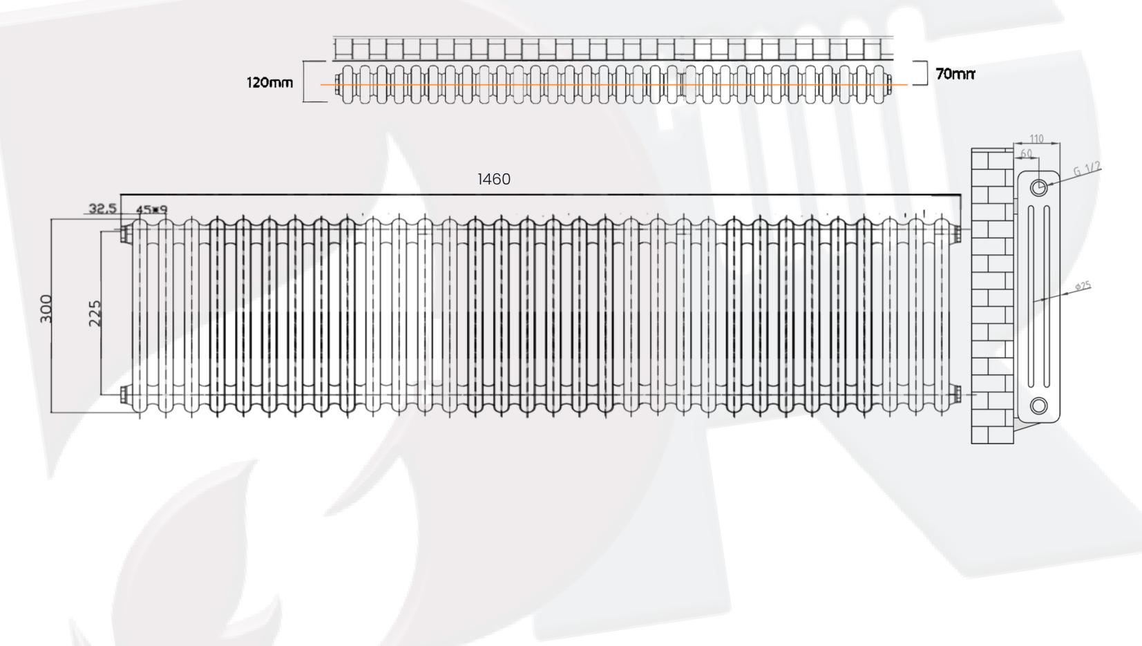
All Direct Radiators are BOE and pipe centres are the radiator width plus 74mm.
